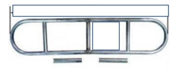
Rear bumper corners to be smooth and capped and cannot be wider than the Rear tires.
